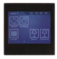
The main interface shows time and date, page name and functional buttons. Slide down the screen, there will be a key scene screen, click on the upper right corner setting button, you can modify the date and time, and on/off timer. Switching pages by sliding around.
