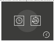
The left icon is used to set the current time and date, the right icon is used to set the timer switch.
